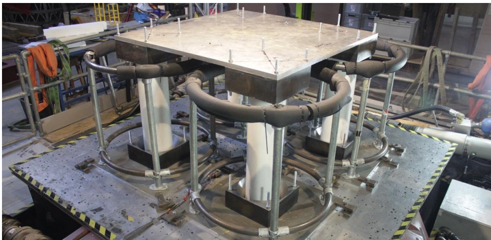
Figure 3: Wobbling specimen on the University of Bristol shake table.
