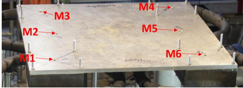
Figure 4: Marker positions on top of the aluminum slab used for wobbling specimen displacement measurements.
